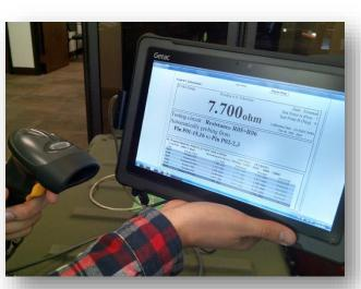
Optional 1D bar code scanner and rugged tablet computer
