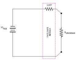
Simplified measurement circuit for safety analysis
