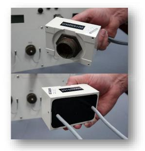
Failsafe connectors are housed in fully sealed potted assemblies
