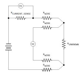
All test circuits use the same fundamental concept. The circuit is constructed of a known precision current sensing resistor in series with the unknown resistor. The processor measures the voltage V1 across the current sense resistor ( $R_{CURRENT.SENSE}$ ) and the voltage V2 across the unknown resistor using a high accuracy differential amplifier. The Ohm's law calculation is
