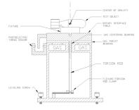
**KSR Series** – These instruments measure moment of inertia and center of gravity with high accuracy.
