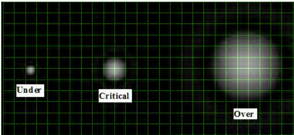
Figure 3. Pixel Grid with Various Examples of Sampling
