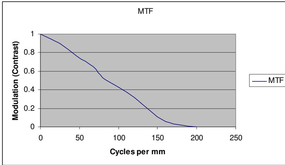
Figure 5. MTF plot of Contrast Ratio versus Frequency of line pairs at the image plane
