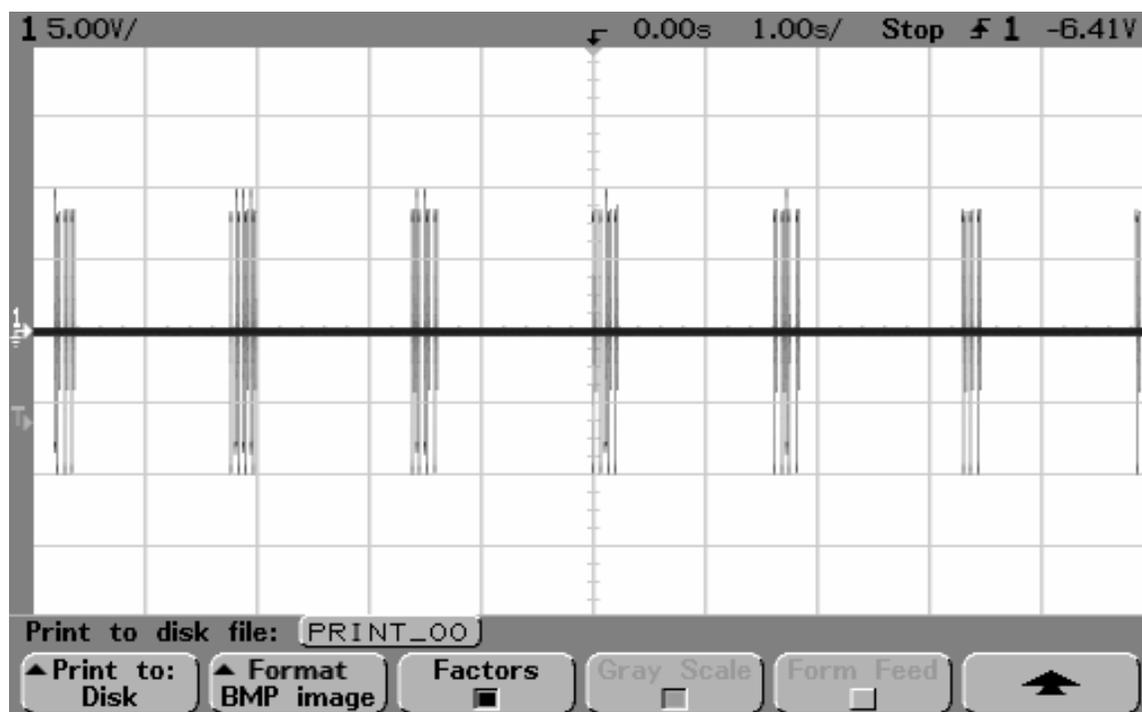
Figure 19. Correction Signal sent to Servo Driver under balanced conditions
