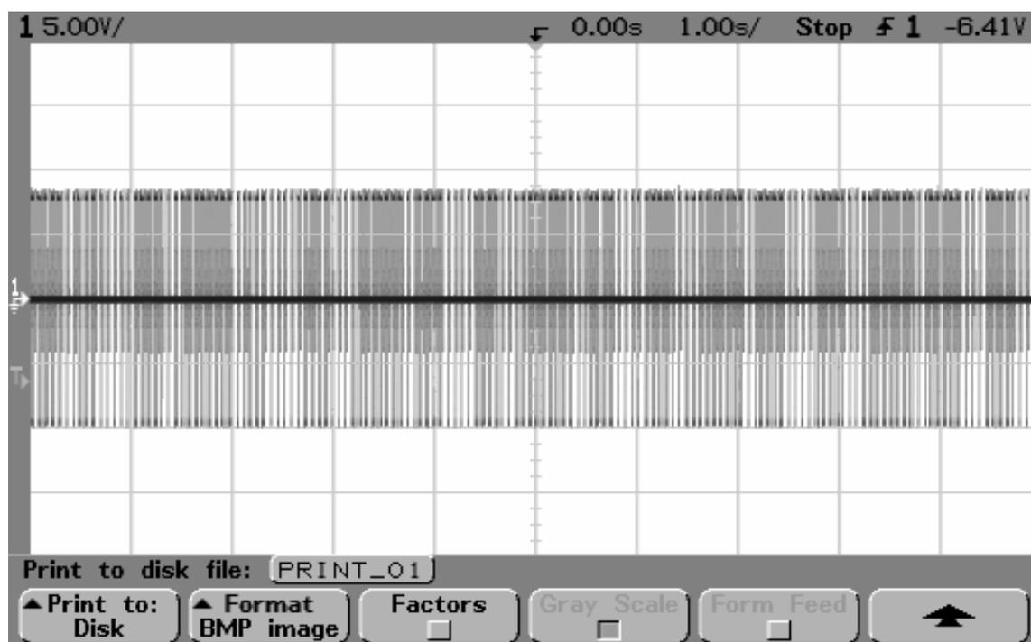
Figure 20. Correction Signal sent to Servo Driver with unbalanced gimbal
