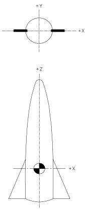
**Figure 15 -** X, Y and Z are principal axes
