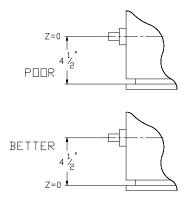
Reference axes must be located at physical points on the object that can be accurately measured. Although the center line of a ring may exist in midair, it can be accurately measured and is therefore a good reference location as can the center of a close tolerance hole which could be identified as the zero degree reference to identify the X axis (Fig. 4).
