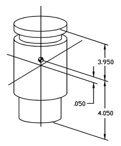
Three mutually perpendicular reference axes are required to define the location of the center of gravity of an object. These axes are usually selected to coincide with edges of the object, accurately located details, or the geometric center of the object.
